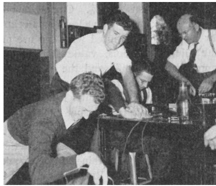
Fig. 9. Subject in process of determining his let-go current and voltage
